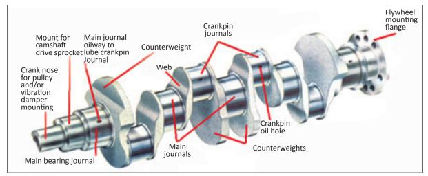
The 3rd main bearing or the center main bearing is where the thrust bearing is located, which ensures that the crankshaft has the proper axial end play. The crankshaft gear on the front end of the crankshaft drives the oil pump and crankshaft balancer. The back of the crankshaft is mounted with a target wheel to send signals to CKP (Crankshaft Position Sensor).
