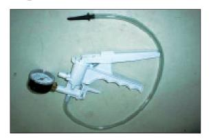
Vacuum pump is used to create vacuum pressure at any component, which works on vacuum and measure the voltage output or functional operation. For inspection of MAP sensor [as shown in the picture] the gauge needs to be connected to with sensor and by creating a vacuum pressure. The output voltage of the sensor is notified on the multimeter.
