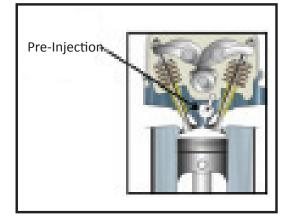
Here fuel is injected into a small pre-injection chamber which is connected to the cylinder by a narrow opening. The initial combustion takes place in this prechamber slowing the rate of combustion
