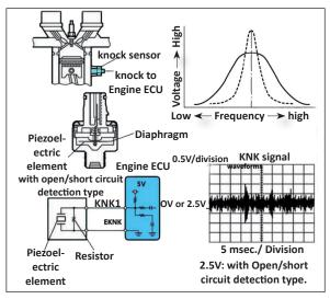
The engine knock frequency is in the range of 6 to 13 kHz depending on the engine model. The proper knock sensor is used in accordance with the knocking generated by each engine
