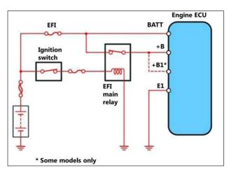
Battery voltage is supplied at all times to the BATT terminal of the engine ECU to prevent the diagnostic codes and other data in its memory from being erased when the ignition switch is turned off.
