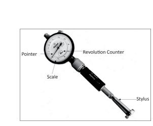
Measurement of engine cylinder bore using bore gauge
