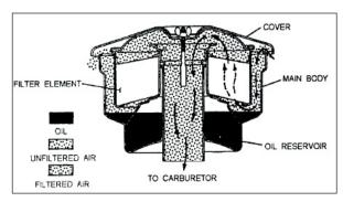
Figure 4-15,-Wet-type air filter
