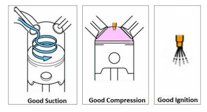
To achieve these elements simultaneously, it is important to precisely control the injection of fuel to create proper combustion and maximum efficiency.
