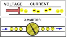
Current can be described as the rate of electron flow. It is measured in amperes. The current increases as pressure or voltage is increased – provided that circuit resistance remains constant. Another term for amperes is 'intensity of current'. The symbol for current intensity is I. The symbol for amperes is A.
