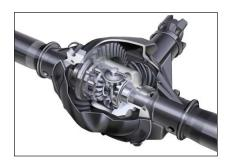
A differential is a gear mechanism that is housed in the transaxle in the case of front wheel drive vehicle or in the rear axle in the case of a rear wheel drive vehicle. The main function of a differential is to differentiate the speed of the inner and outer wheels while on a turn to prevent skidding.
