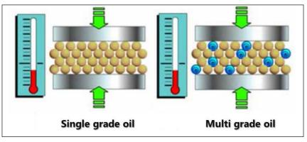
An example of multi-viscosity lubrication oil is as below:
