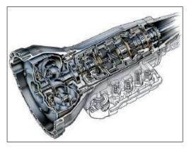
Transmission is a solid robust device that is made up of gears of different sizes mounted on parallel shafts. It is situated between the clutch and the driveshaft in the case of a front wheel drive vehicle and clutch and the propeller shaft in a rear wheel drive setup. It works on the principle of gearing, in which a set of gears mesh together to provide the desired output speed. The output speed also depends on the gear ratio of the meshing gears.
