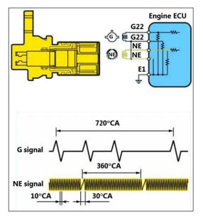
The engine ECU uses the NE signal and G signal to calculate the basic injection duration and basic ignition advance angle. As with the G signal, the NE signal is generated by the air gap between the crankshaft position sensor and the protrusions on the NE timing rotor periphery installed on the crankshaft. The illustration shows a type of signal generator with 34 protrusions on the NE timing rotor periphery and an area with two teeth missing.
