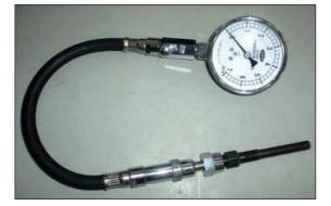
Compression gauge is used to measure the compression pressure
