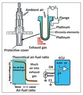
At high temperatures (400°C [752°F] and higher), the zirconium element generates a voltage as a result of the large difference between the oxygen concentrations on the inside and outside of the zirconium element.
