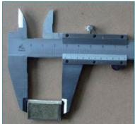
Stylus is provided to measure depth, internal jaws to measure internal dimensions and external jaws to measure external dimensions.
