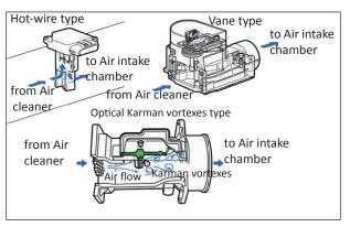
Currently, most models use the hot-wire type of air flow meter because it has superior measurement accuracy, lighter weight, and better durability.
