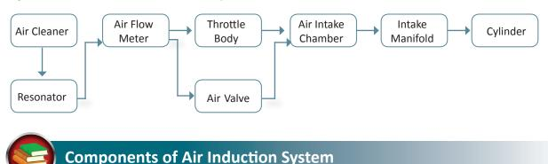
A general schematic of an air induction system is as below.
