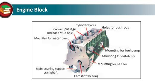
An engine block is made up of cast iron or aluminum. It is the main component of an engine as all 4 strokes or cycles are carried out in it. Like the cylinder head, engine block also has coolant passages, lubrication passages, galleries, exhaust and intake etc. machined in it. It consists of cylinder bores and provisions for the crankshaft and other sub components fitments
