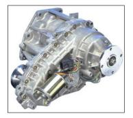
A transfer case is generally seen in vehicles equipped with four wheel drive system. It is connected to the transmission and also to the front and rear axles by means of drive shafts. Its primary function is to transfer power to the front as well as the rear when the four wheel drive is engaged.
