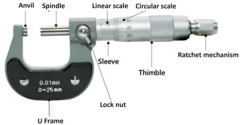
Dimension = Linear scale reading + Circular scale reading + Zero error reading
