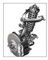
Suspension system isolates the cabin from the road shocks to provide comfortable drives. Automobiles are generally equipped fully independent suspension setup in the front and semi-independent or non-independent suspension at the rear. Recently automobiles are also equipped with all independent set-ups too.
