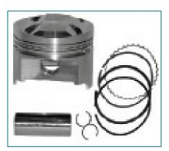
Usually three in numbers and the top two are compression rings and the bottom helical one are oil rings. The piston pin is made up of steel and has two locks to keep the piston in place and connected to the connecting rod.
