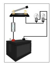
The parallel circuit has two or more paths for electrons to flow. Current in this circuit is shared between the branches.
