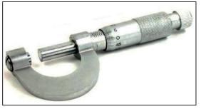
Micrometer to get the precise reading. The ratchet at the end helps rotating the barrel and the spindle. As soon as the job is firmly held between the spindle and the anvil, the ratchet starts slipping thus allowing exerting an even pressure while measuring a component.
